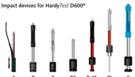
Impact device D: Universal device for most hardness requirements
