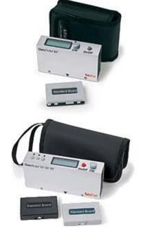
These instruments can be supplied in one and three-angle design. The GlossTector® 60° is equipped with a universal angle of 60° and determines universal and normal gloss levels. The GlossTector®20°-60°-85° determines – depending on its setting – the respective levels for high gloss, universal, normal or dull gloss.
